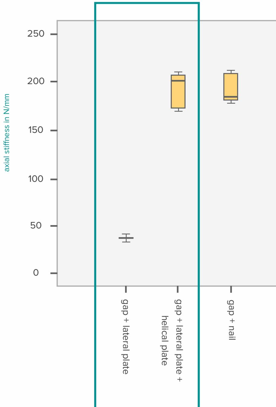
**Fig. 3:** Testing axial stiffness under gap conditions: An eccentric axial load of 100 N was applied. A significant improvement of axial stiffness from lateral plate alone from 36 N/mm to 193 N/mm with additional helical plate was achieved (Mark Lenz et al. AO Research Institute).
