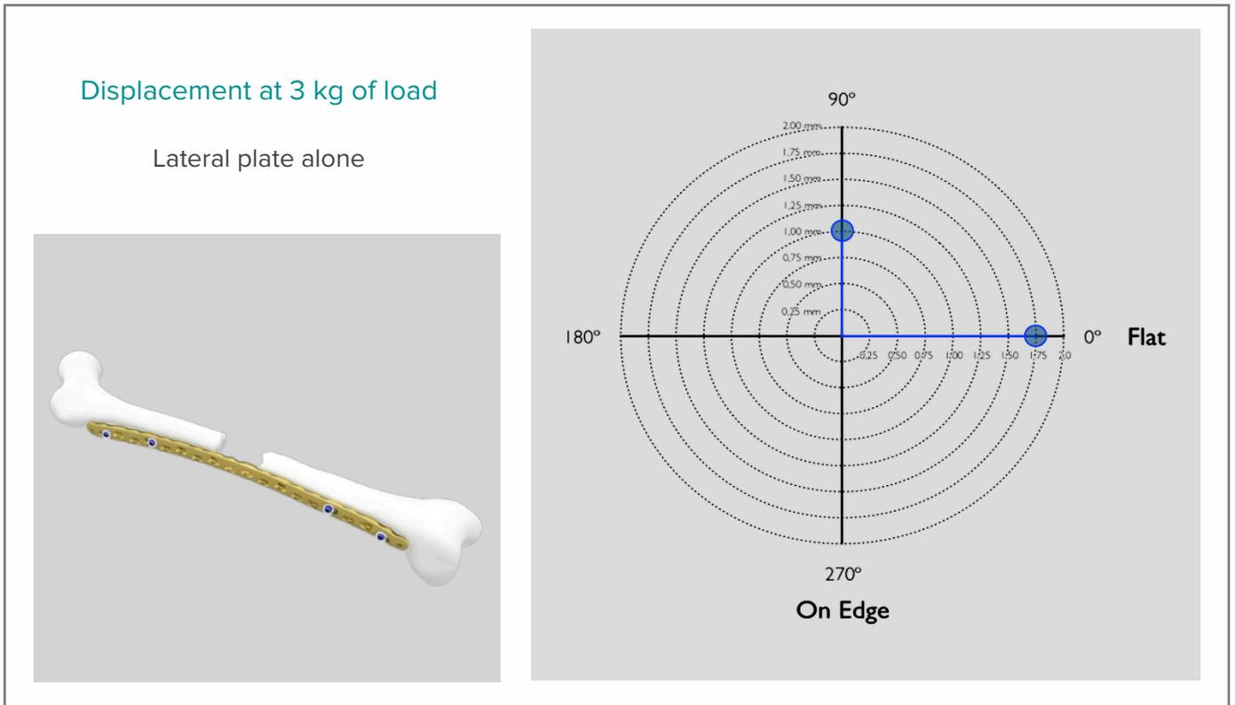
**Fig. 1: Quick and dirty bending test measuring the change of the width of the open fracture gap.** Testing a single lateral plate spanning the gap. The diagram shows a large *stiffness* when the bending is applied around an axis at 90° offset from the flat surface (“*On Edge*”) of the plate and show less stiffness when bending is applied around an axis parallel to the flat surface of the plate (“*Flat*”).
