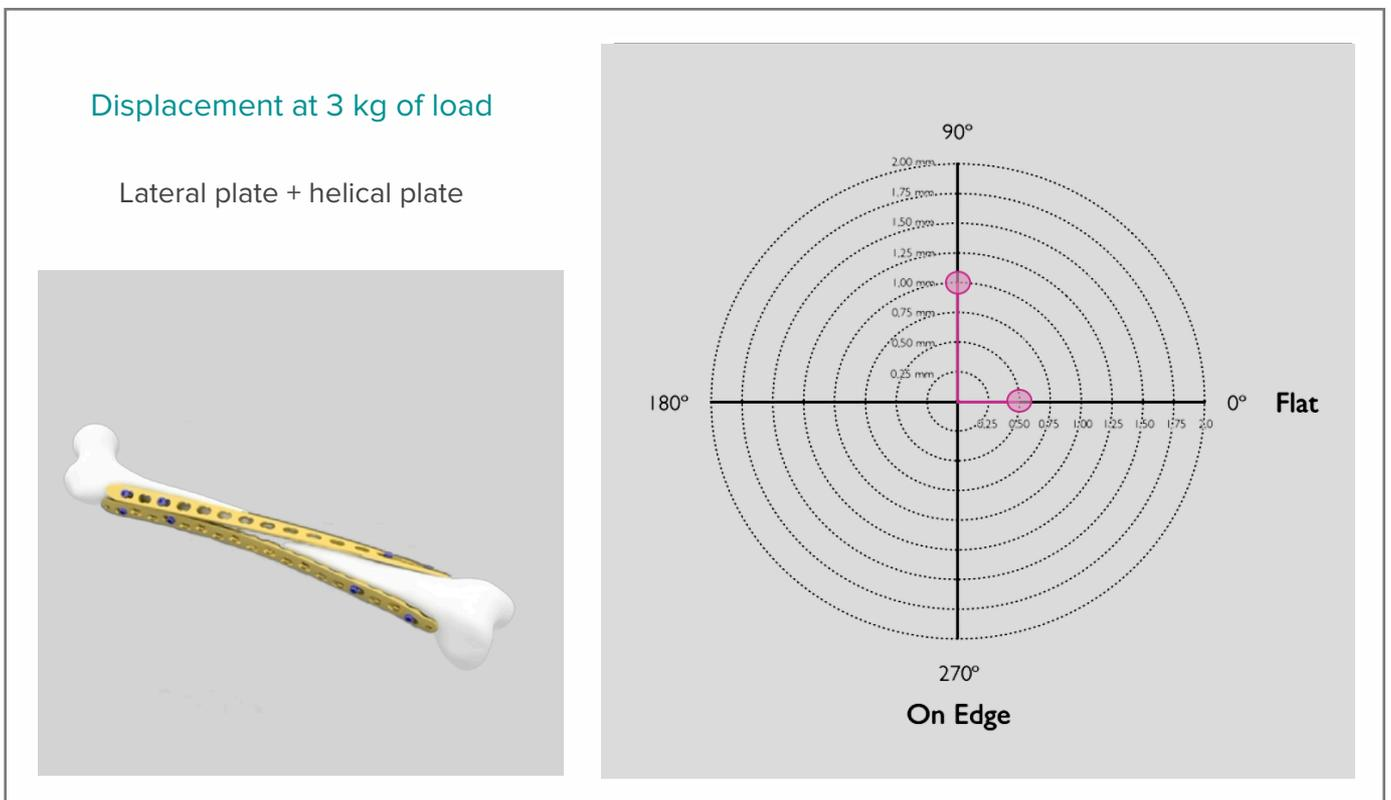
**Fig. 2: Quick and dirty testing of the contribution of the helical plate to stiffness as tested in Fig. 1.** The helical plate improves stiffness when tested around an axis parallel to the flat surface of the plate (“*Flat*”) while when tested around an axis perpendicular to the flat surface (“*On Edge*”), where the initial stiffness is large no additional effect is observed.
