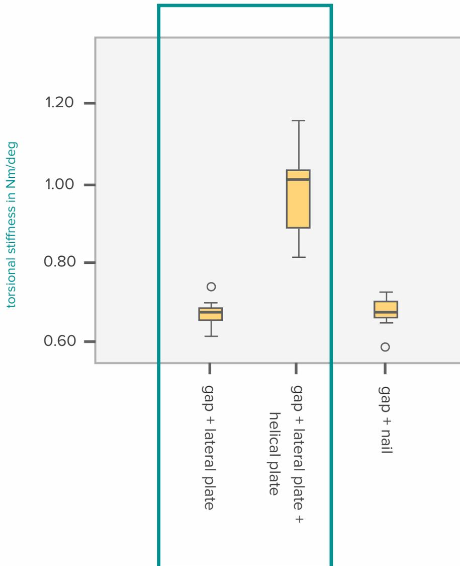
**Fig. 4:** Testing torsional stiffness under gap conditions: A torque of 2 Nm was applied. A significant improvement of torsional stiffness of lateral plate alone from 0.71 Nm/deg. to 0.91 Nm/deg. with additional helical plate was achieved (Mark Lenz et al. AO Research Institute).
