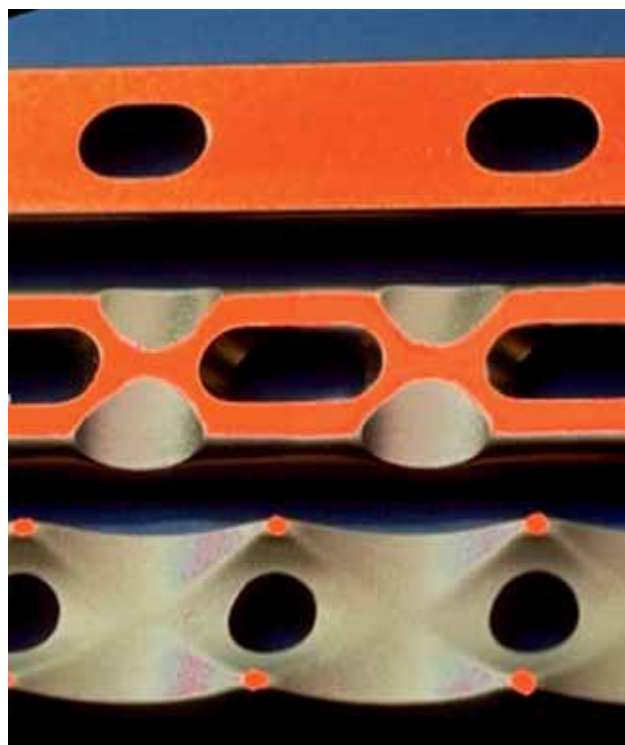
Fig. 3. Minimizing contact damage. - DCP (16) no undercuts, - LC-DCP undercuts, - PC-Fix only point contact
