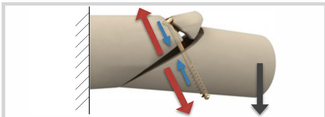
**Fig. 4B** Lag screw positioned near thin end of bone fragment. The bone spike does not resist and breaks, the fracture opens. The function of the lag screw is lost.
