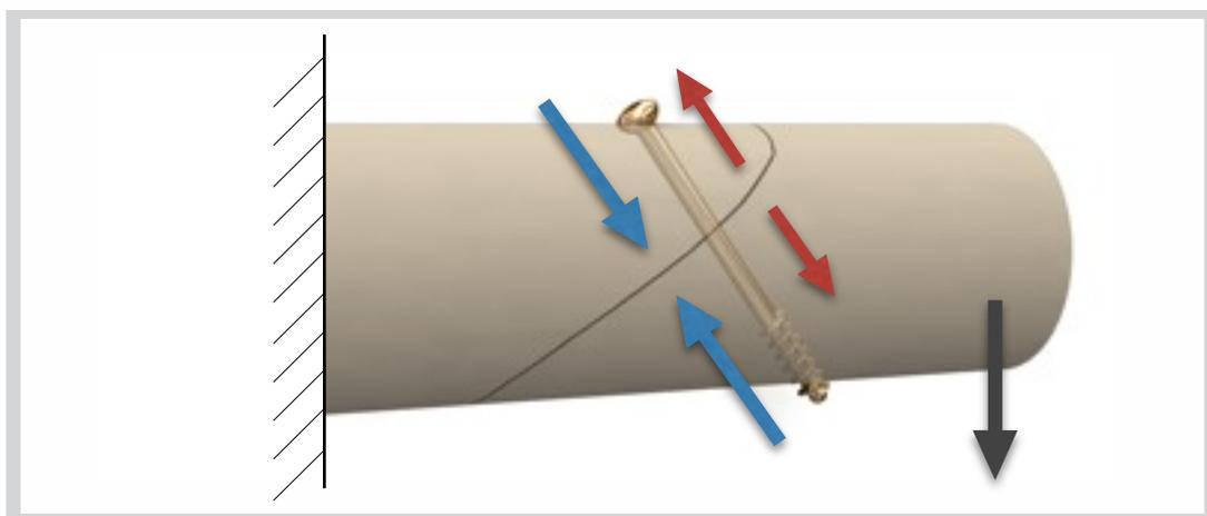
**Fig. 2B Lag screw, balance of forces.** The oblique fracture is stabilized with a lag screw. The compression exerted by the lag screw (blue) exceeds the traction (red) produced by bending. The fracture remains in close contact.
